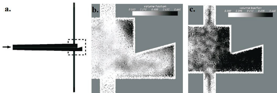
Fig. 2-8. Schematic of Powder Injection Molding and the results
