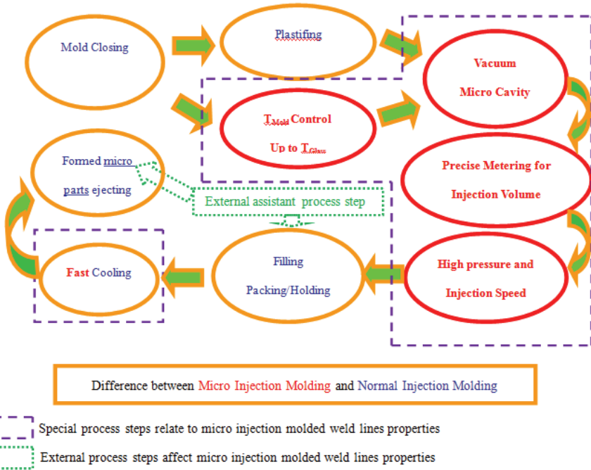
Fig. 1-2. Micro injection molding processing steps
