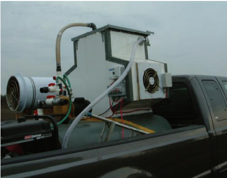
Fig. 1. The odour generator carried on a truck to be positioned at specific distances upwind from the windbreak (Lin et al., 2006)
